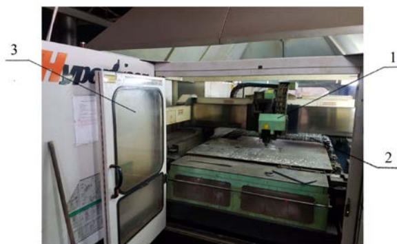
Fig:1 External appearance of the HYPER-GEAR-510 laser cutting complex: 1 - laser machine module; 2 - pallets; 3 - the door closing the work area
